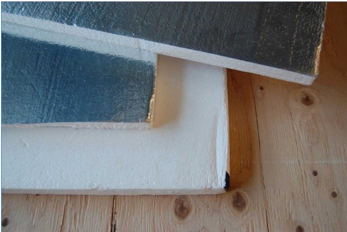
Figure 7. EPS samples with reflective facers (top) and with facing removed (lower) over plywood.
