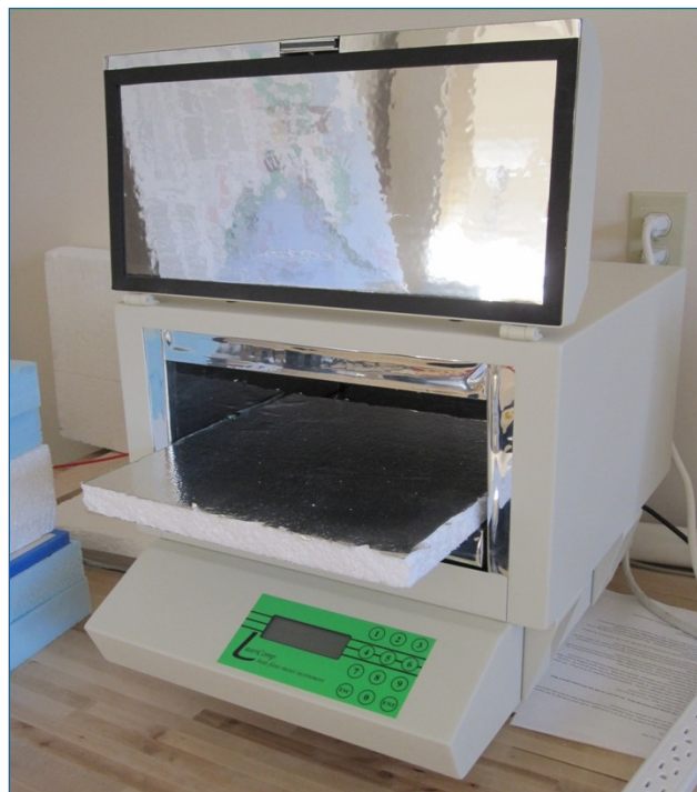
Figure 8. FOX-314 heat flux meter with a one-inch thick EPS sample between the plates. The heat flux meter tests the material for its thermal conductivity by maintaining a temperature difference across the sample and monitoring the energy required to maintain that temperature difference.
