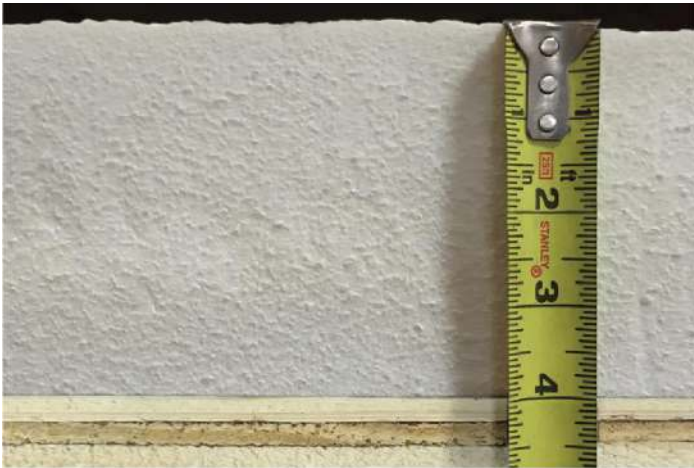
Single lift, high R-value: achieves R-28 in one pass at 4"
