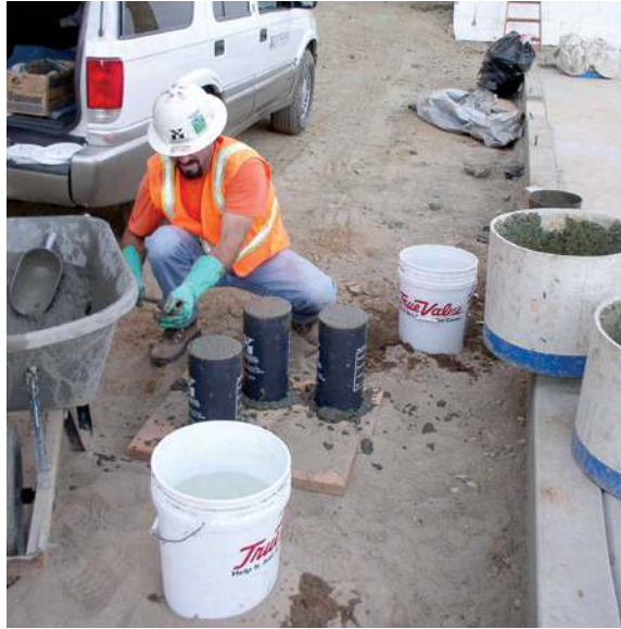
Figure 8.2 – Preparing concrete cylinders for testing
