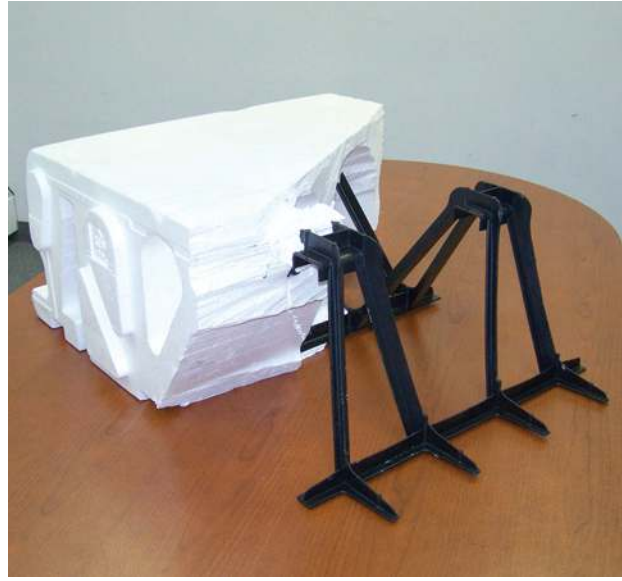
Figure 1.3 – Propylene Web embedded in EPS
