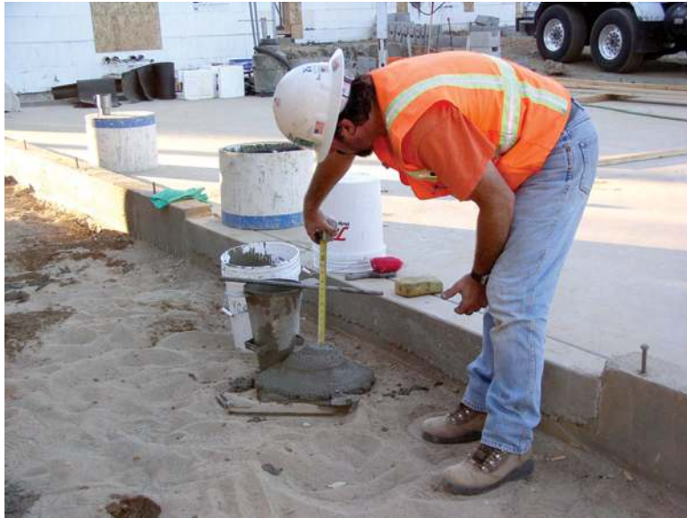
Figure 8.1 – Measuring concrete slump
