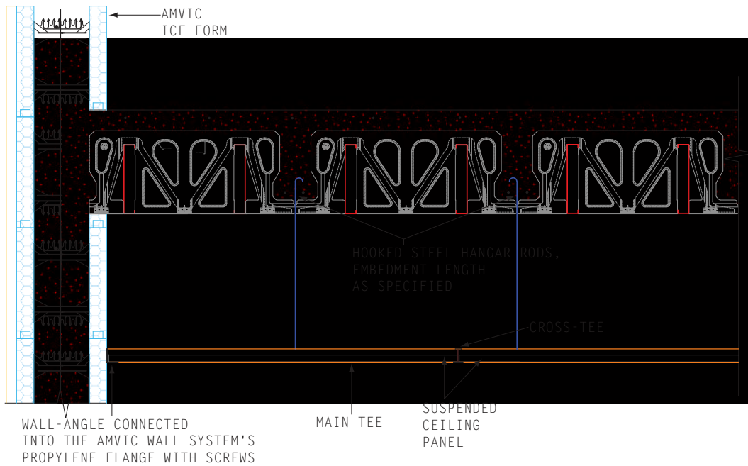
Figure 9.3 - Attaching drop ceiling to concrete joists with hooked steel hanger rods
