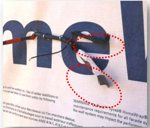
Figure 6. Temperature (black) and humidity (white) sensors were installed on the interior side of air barrier system (taped sheathing, left photo) and on exterior side of air barrier system (right photo).
