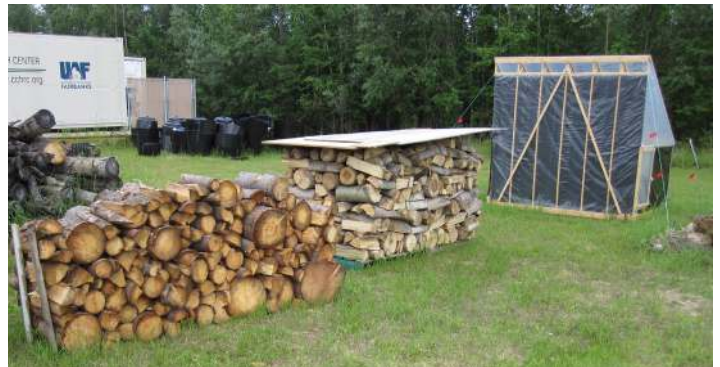
The study tested four storage methods, from left to right: uncovered, simulated wood shed, solar kiln, and covered with a tarp (not pictured).
