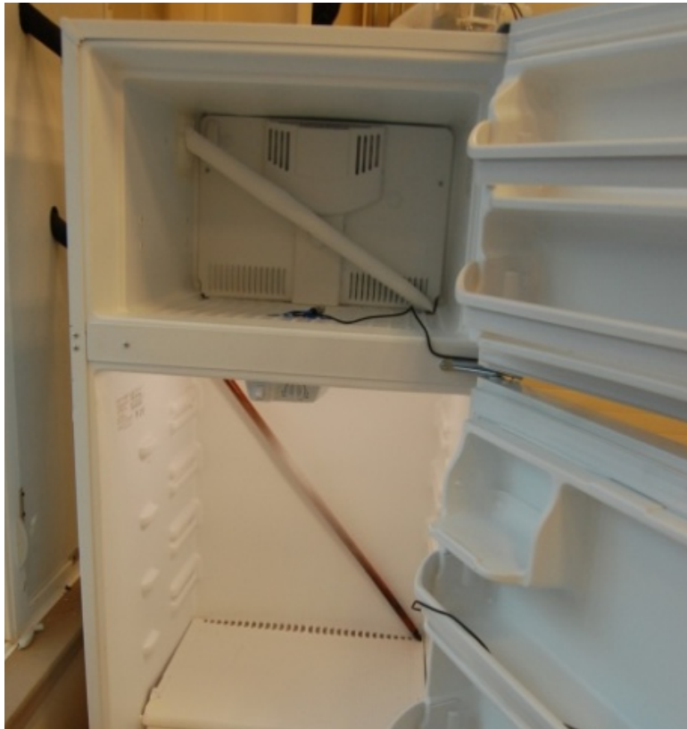
Figure 5. Tubing in the back of the retrofit fridge. The ice build-up on the pipes was not addressed in this study but will probably need to be addressed in future work.
