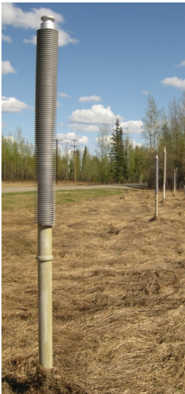
Figure 2. Ground cooling thermosyphons. Test thermosyphons in front of CCHRC are being monitored to further understand their performance.
