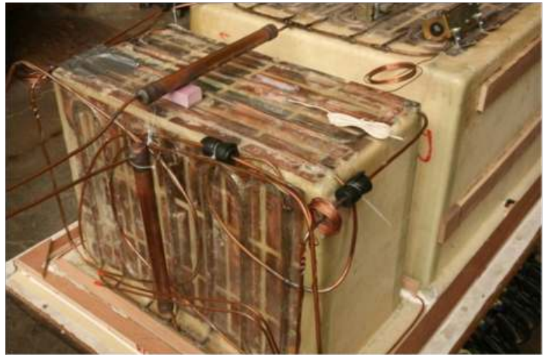
Figure 17. The Sun Frost prototype showing the interior tubing. This picture shows the backside of the freezer compartment in the foreground and a portion of the refrigerator compartment toward the back.
