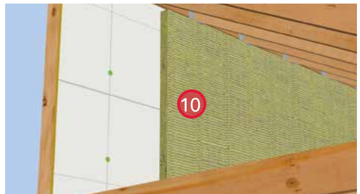
10. Install ROCKWOOL COMFORTBOARD™ 80 on the exterior of the wall between canopy ledger boards with recommended fasteners.
