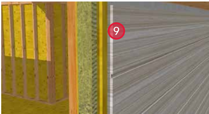
9. Install cladding. Provide venting at the top of the wall to allow for the free movement of air through the wall cavity. It is not recommended to vent the wall cavity into the roof.
