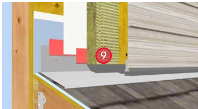
9. Install cladding and closure flashing.
