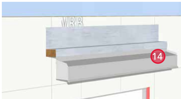
14. Install self-adhered membrane over the wood blocking. Extend the membrane onto the adjacent wall and the prefinished metal flashing.
