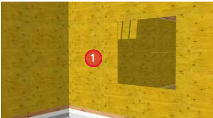
1. Typical wood frame construction at sheathing stage.
