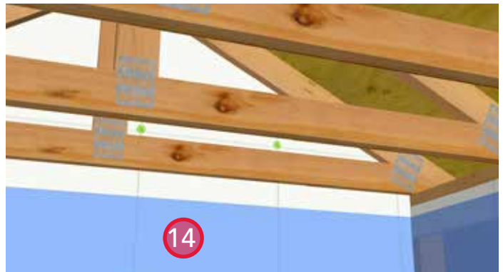
14. Install poly on the walls and fasten to the sheathing membrane with staples.
