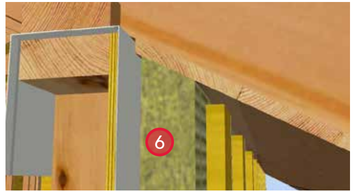
6. Install ROCKWOOL COMFORTBOARD™ 80 and strapping to the exterior of the wall. Provide bugscreens at the top and bottom of the strapping.
