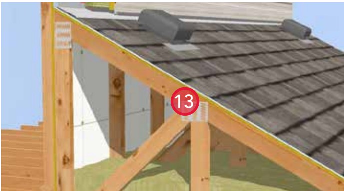
13. Install ROCKWOOL COMFORTBATT® in the attic space. Insulate wall adjoining attic space and occupied space with ROCKWOOL COMFORTBATT®.
