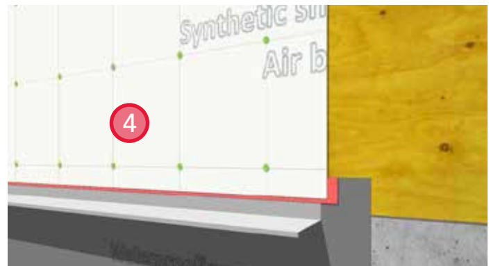
4. Install sheathing membrane and seal leading edge with sheathing tape to complete air barrier continuity. Provide a \frac{3}{4} " vision line on the flashing backleg.
