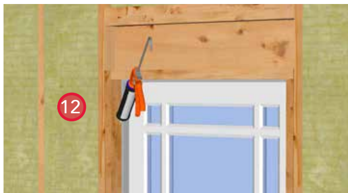
12. Install backer rod and sealant around the interior perimeter of the door frame to maintain air barrier continuity.
