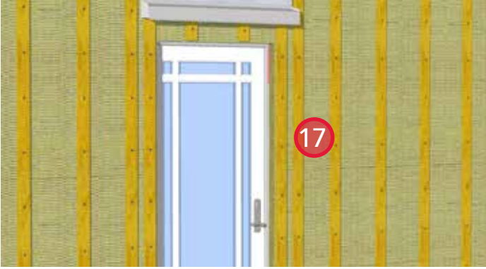
17. Install ROCKWOOL COMFORTBOARD™ 80 and secure in place with strapping. Provide bugscreens at the bottom and top of the strapping.
