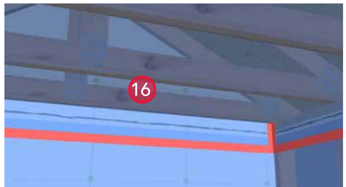
16. Install poly to the underside of the roof framing and fasten with staples at the sealant bead to complete the air seal. Seal the leading edge with sheathing tape.
