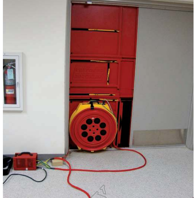
A blower door test can help determine air leakage.
