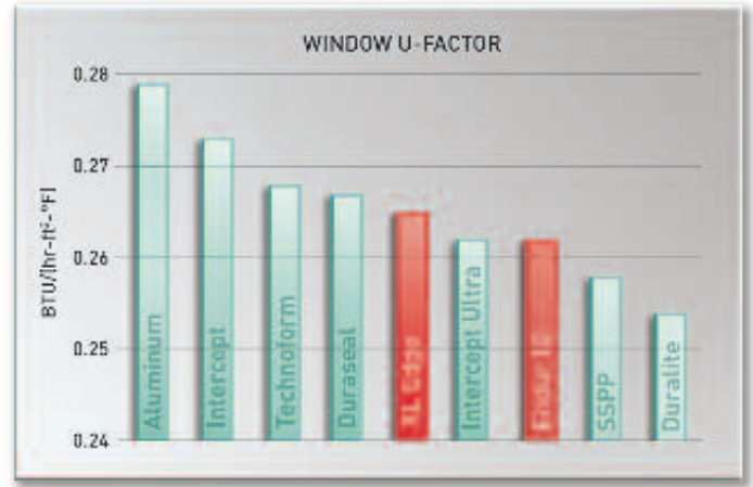
1) 3.1 mm LoE 3 -366 / 0.5" Argon / 3.1 mm Clear 2) Generic Wood / Vinyl Frame
