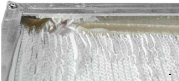
Membrane detaches in the corner, breaking the seal.
