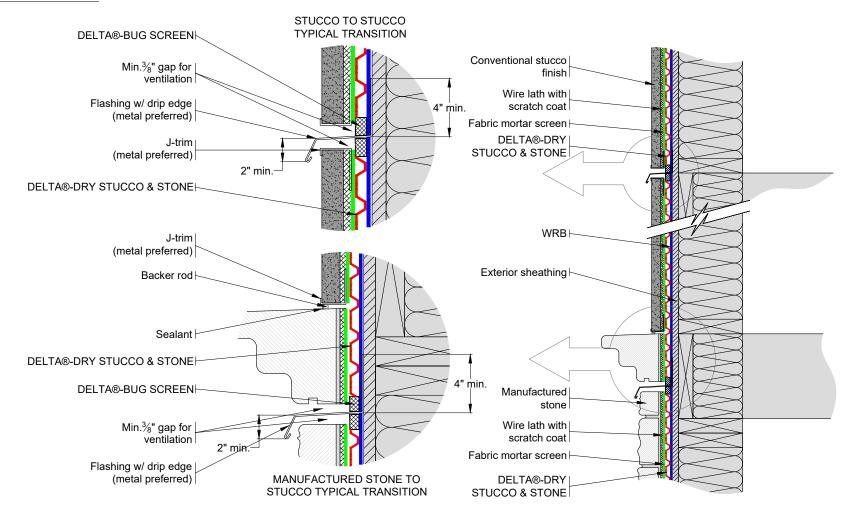
\*\*For proper performance of DELTA®-DRY ensure top and bottom remain open to allow ventilation and drainage\*\*
