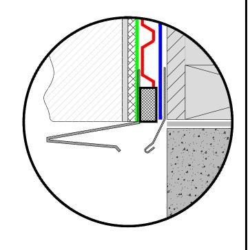
\*\*For proper performance of DELTA®-DRY ensure top and bottom remain open to allow ventilation and drainage\*\*
