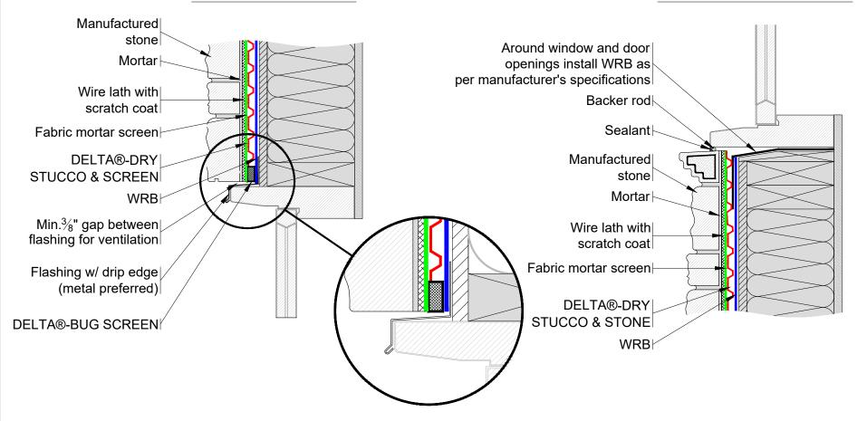
\*\*For proper performance of DELTA®-DRY ensure top and bottom remain open to allow ventilation and drainage\*\*
