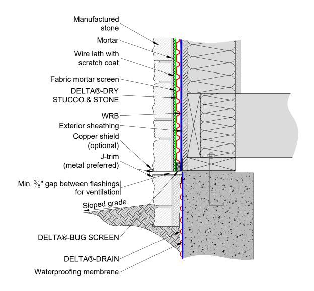
\*\*For proper performance of DELTA®-DRY ensure top and bottom remain open to allow ventilation and drainage\*\*
