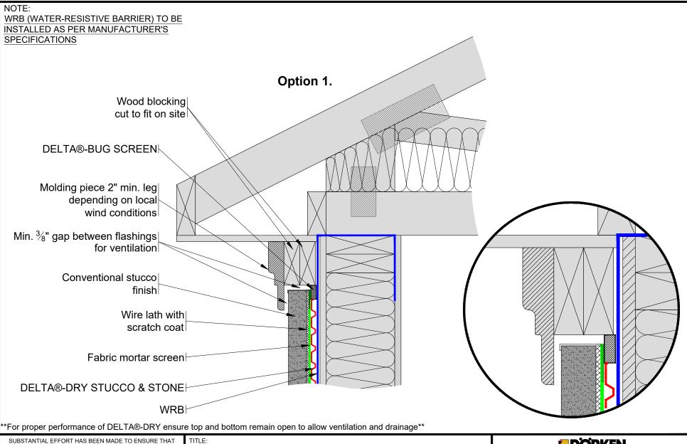
DELTA®-DRY STUCCO & STONE RAINSCREEN APPLICATION WITH CONVENTIONAL STUCCO FINISH TOP OF WALL DETAIL OPTION 1
