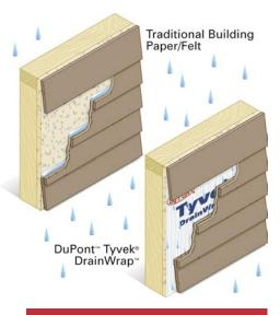
The drainage component of DuPont<sup>\*</sup> Tyvek<sup>\*</sup> DrainWrap<sup>\*</sup> helps keep out bulk moisture and air, helps protect insulation, and helps prevent the formation of unhealthy mold and mildew.
