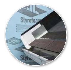
**STEP 3** Place first shingle and next section of sidewall flashing over up-slope edge of diverter, lapping a minimum of 4" over diverter.
