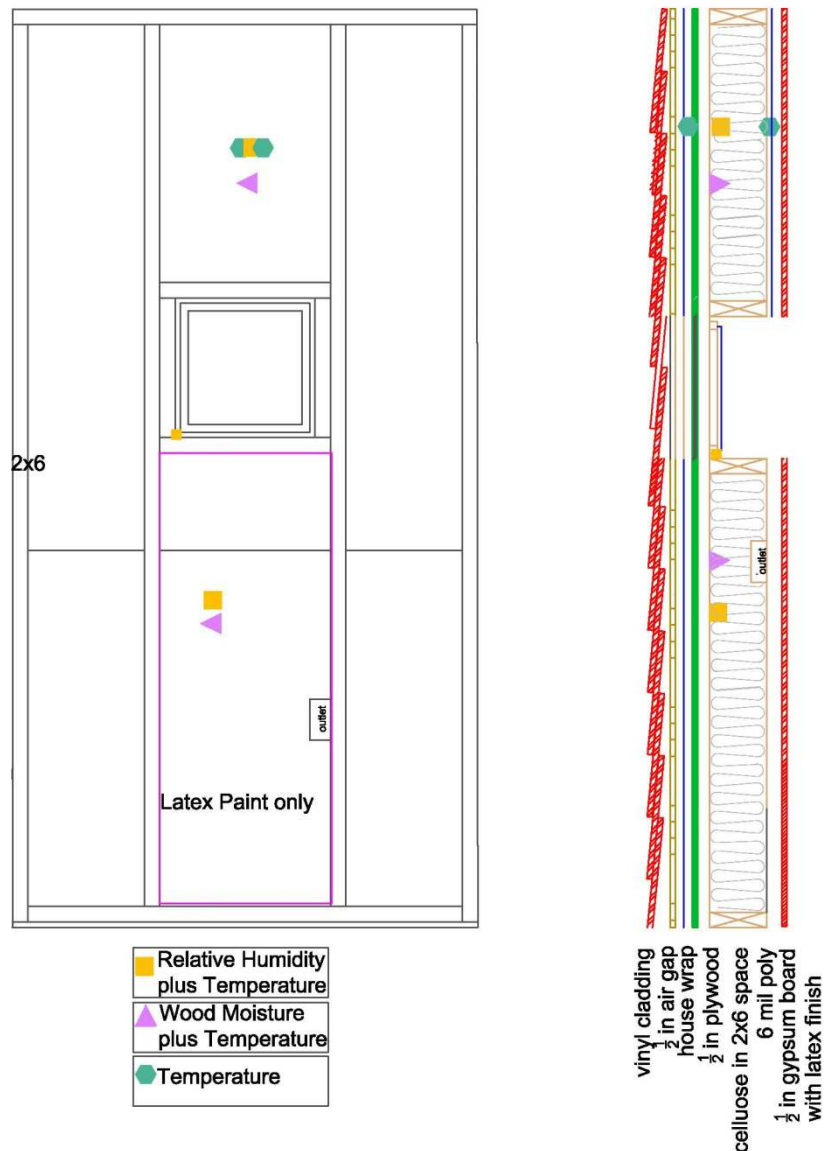
Figure 7. The cellulose wall. All of the wall but the space below the window had a 6 mil vapor retarder.
