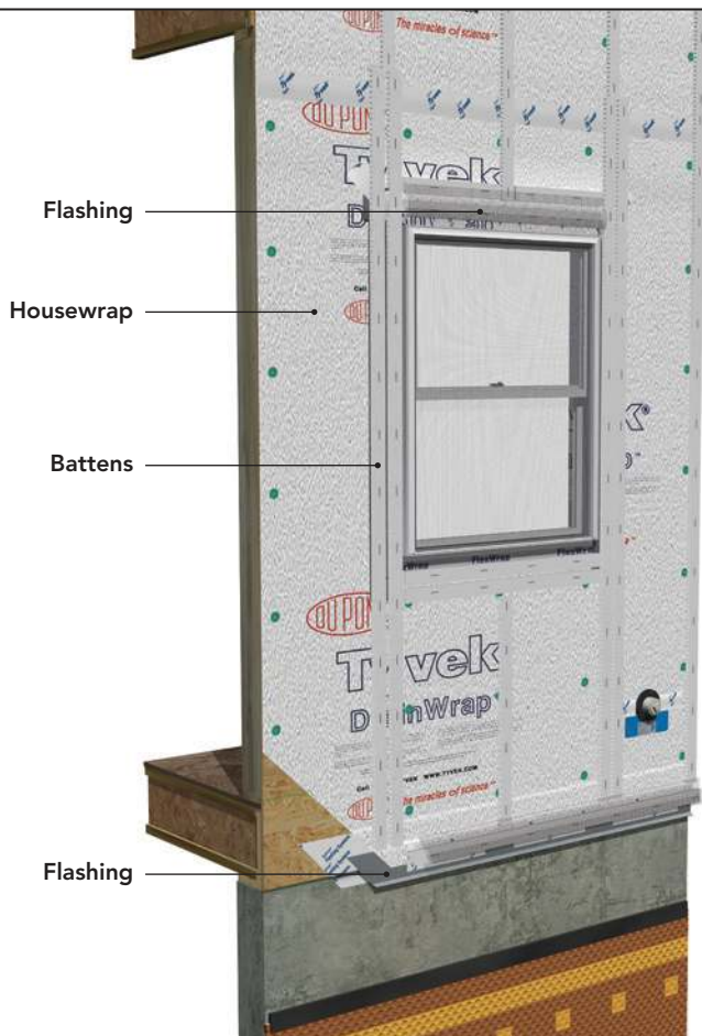
FIGURE 1: WINDOW INSTALLED TO SHEATHING
