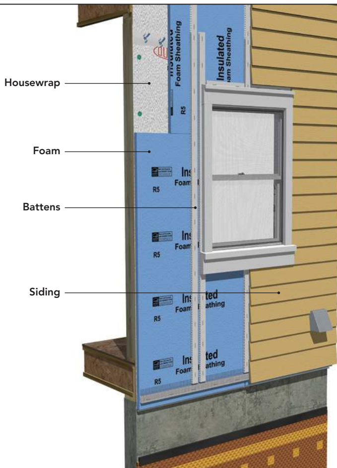
FIGURE 2: WINDOW INSTALLED TO FOAM
