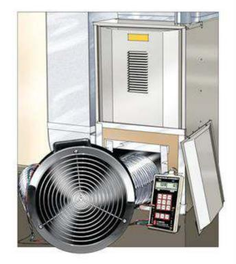
Performance testing is critical for right-sized HVAC systems, since they're operating within a narrower margin of error in terms of design calculations. Tight ducts and air-handling equipment are keys to overall performance, so make sure to run duct blaster tests to assure air leakage rates of 3% or less of gross air flow.
