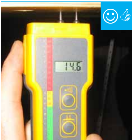
A moisture meter verifies that the moisture content of the framing is below the recommended 18%.
