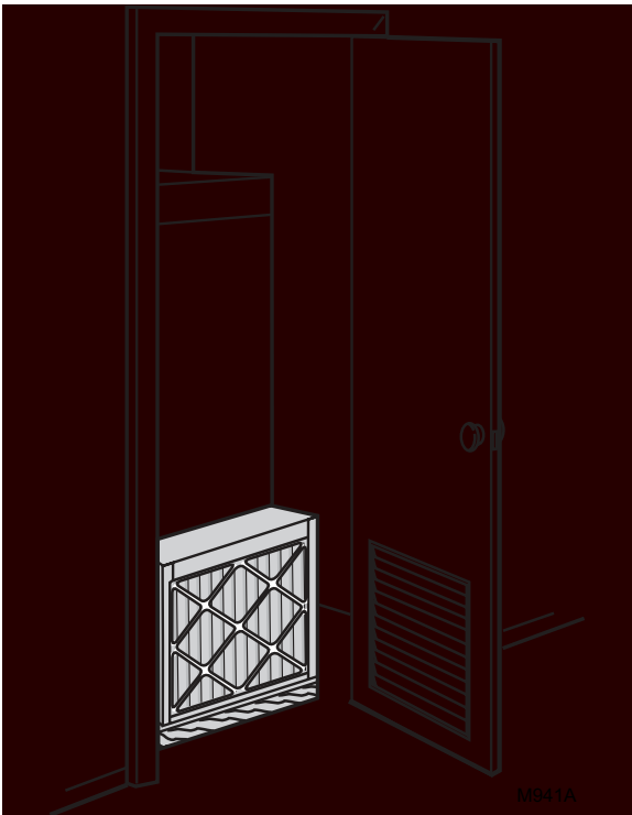
Fig. 3. Highboy furnace, with closet installation. Electronic Air Cleaner is mounted vertically on furnace between furnace and louvered return air opening in closet door.
