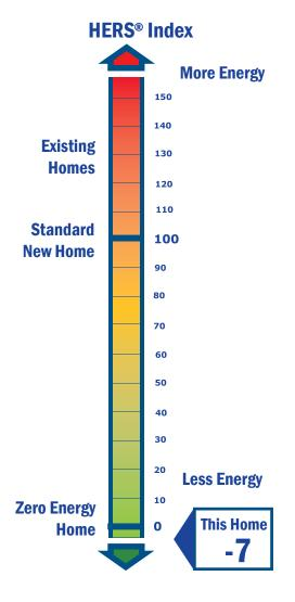
As specified in the Challenge Home requirements, the envelope was designed to meet all ENERGY STAR Version 3 requirements and 2012 International Energy Conservation Code (IECC) insulation levels. Final blower door tests confirmed a tight envelope at 1.77 ACH 50.
