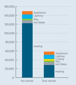
This chart shows the projected site energy savings resulting from the heat pump installation, as modeled in Energy Gauge.
