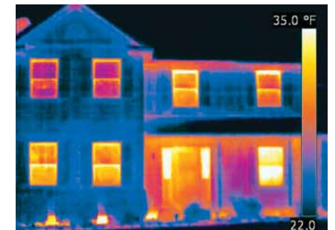
Evidenced in the blue areas above, continuous insulation greatly reduces energy loss by preventing it from leaking out of walls.
