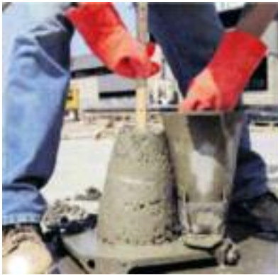
Figure 10.4 - Concrete mix with low slump. ©2006 Cement Association of Canada, EB 101-7 figure 16-2
