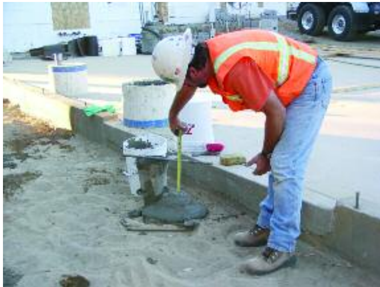
Figure 11.5 – Performing the slump test in the field
