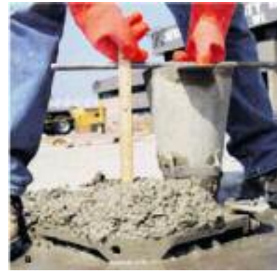
Figure 10.5 - Concrete mix with high slump. ©2006 Cement Association of Canada, EB 101-7 figure 16-2
