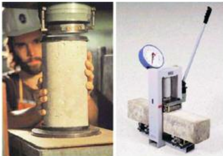
Figure 10.3 - Testing the concrete cylinder for compressive strength (left) and concrete beam for flexural strength (right). ©2006 Cement Association of Canada, EB101-7 figure 16-15
