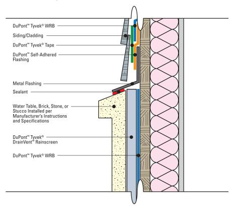
Option 2: DuPont™ Tyvek® DrainVent™ Rainscreen Installed Behind Siding/Cladding and Lower Facade
