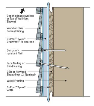
Install wood siding or fiber cement cladding over DuPont™ Tyvek® DrainVent™ Rainscreen in accordance with the cladding manufacturer's recommendations.
