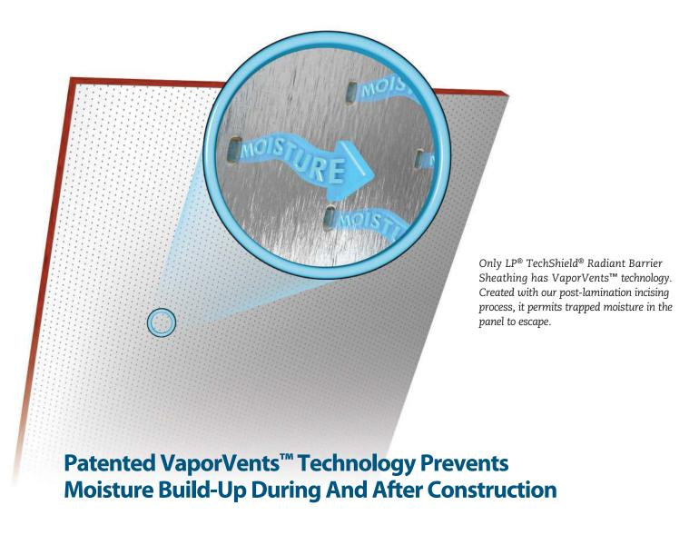
Only LP TechShield sheathing features VaporVents<sup>™</sup> technology. Created with our patented post-lamination foil incising process, it allows LP TechShield panels to dry more quickly than other radiant barrier panels when moisture occurs during construction. It also allows for continued moisture evaporation after installation. No other brand of radiant barrier sheathing offers this unique, important feature.
