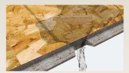
The RainChannel self-draining notch system allows water to drain quickly from the surface. Combined with a moisture-resistant edge seal, the RainChannel system helps fight moisture absorption and edge swell, reducing the need for sanding.
