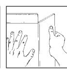
Snap board along the score over the edge of a solid support. (A quick action produces the best results.)
