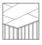
Start with proper framing. Be sure studs are straight to provide adequate nailing surface at adjoining walls.
