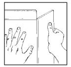
Snap board along the score over the edge of a solid support. (A quick action produces the best results.)
