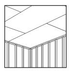
Start with proper framing. Be sure studs are straight to provide adequate nailing surface at adjoining walls.
