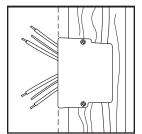
Align all electrical outlets, heating ducts, etc., so they will be flush with the drywall surface.
