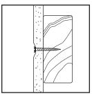
Slightly recess the nail or screw head. Indent face paper without tearing it.
