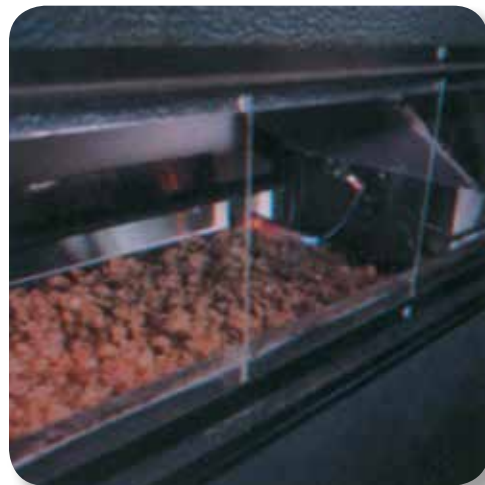
Fiber glass loosefill and batt insulations pass the ASTM E970 fire safety test.
