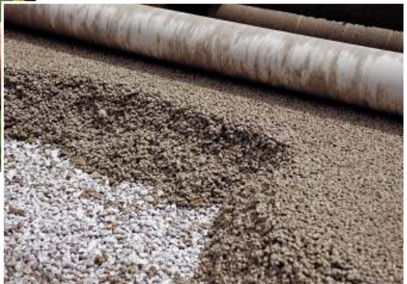
Figure 1. Made largely without fine aggregates, pervious concrete has a porous structure that allows up to 18 gallons of water per minute per square foot to flow through it — yet the material can have a compressive strength of more than 3,000 psi when fully cured.
