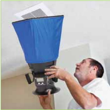
Balometer used to verify installed performance
