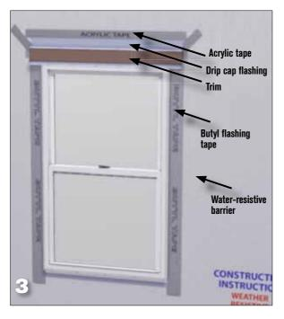
While there is still ongoing debate about the best way to flash a window with an integral nailing flange, peel-and-stick flashing tape or adhesive membrane, peel and stick butyl adhesive flashing tape is a commonly accepted approach to ensure the continuity of the drainage plane when a weather resistive barrier is part of the wall assembly.
