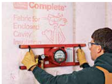
Inspect-R® Density Gauge accurately reads R-values in seconds.
