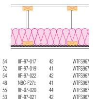
Wood truss floor, trusses utilizing framing members not less than 38 mm x 89 mm (1-1/2" x 3-1/2"), spacing and depth as specified below, 15.5 mm (5/8") OSB subfloor, resilient channels spacing specified below, single layer 15.9 mm (5/8") type "x" gypsum board ceiling finish; 152 mm (6") thickness EcoTouch® QuietZone® PINK™ FIBERGLAS® Acoustic Batt Insulation.
