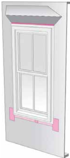
Step 11: Fold housewrap down at head. Ensure head flap has not been damaged during the installation process.
