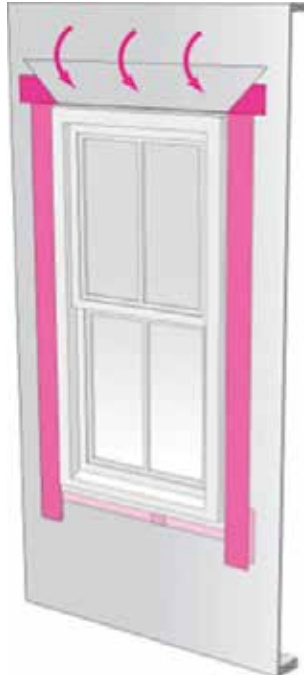
Step 8: Install window plumb, level and square per manufacturer's instructions.
