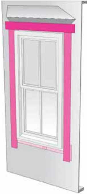
Step 7: Back-caulk window. Apply sealant at jambs and head; do not apply to sill to allow for drainage. Or, caulk can be applied to window nailing flange prior to installation.
