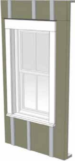
Step 19: Trim installed at head and jambs; sloped cap flashing (shown) installed over lower trim at head of window.
