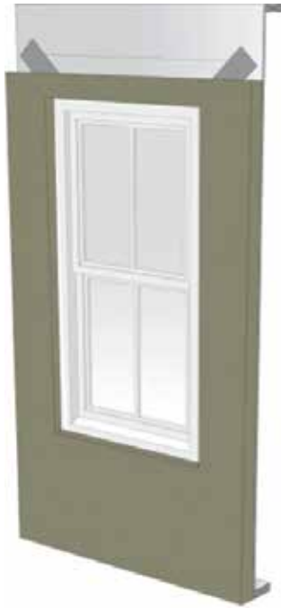
Step 13: Install ROXUL COMFORTBOARD IS insulation.
