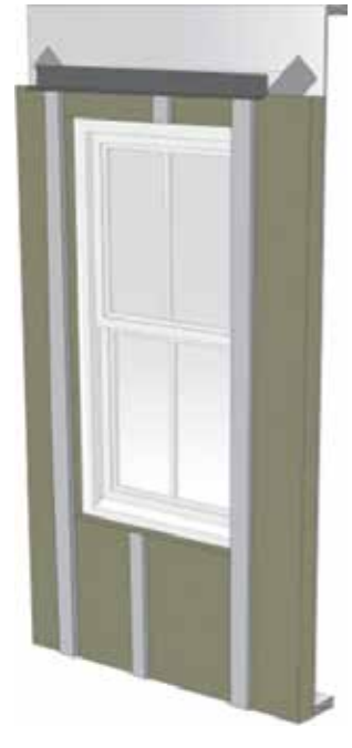
Step 15: Outward leg of cap flashing extends past face of trim (to be added in Step 19).
