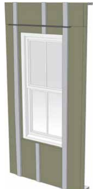
Step 18: Install next course of ROXUL COMFORTBOARD IS and furring. Drainage gap created by furring. Do not fasten furring through head cap flashing.
