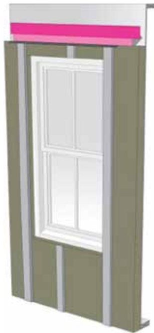
Step 17: Sheathing tape applied over adhesive membrane strip to secure top edge.
