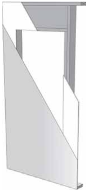
Step 1: Wood frame wall sheathed with OSB or plywood with housewrap as drainage plane.
