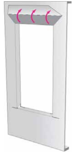
Step 3: Housewrap folded in at jambs and sill and secured tightly. Head flap folded outward; or, tuck head flap under.
