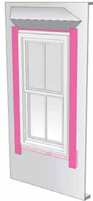
Step 12: Apply corner patches at head; extend minimum 1" beyond cut in housewrap. Air seal window around entire perimeter on the interior with sealant or non-expanding foam.
