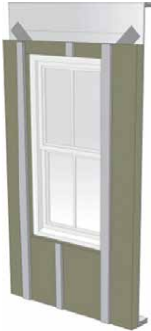
Step 14: Install furring over ROXUL COMFORTBOARD IS insulation.
