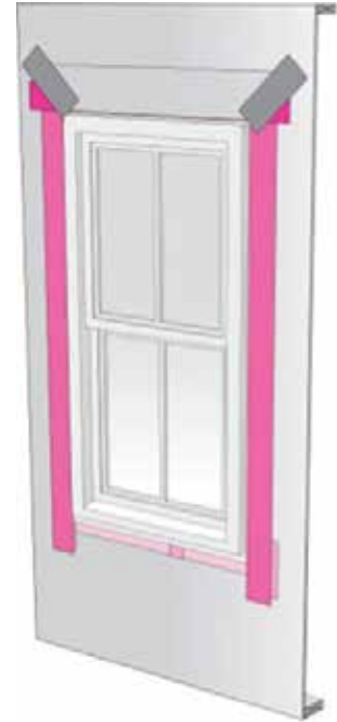
Step 9: Install jamb flashing; extend minimum 1" above head nailing flange and a minimum 3" below sill nailing flange.
