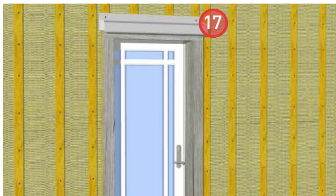
17. Install metal flashing to the strapping above the top trim board to aid in water diversion.
