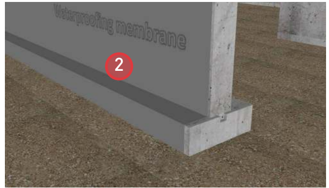
2. Install the below-grade waterproofing membrane. Ensure the membrane wraps over the footing and terminates on the vertical.
