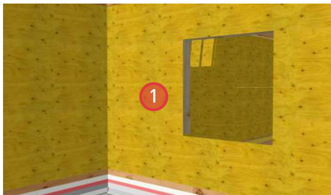
1. Typical wood frame construction at sheathing stage.
