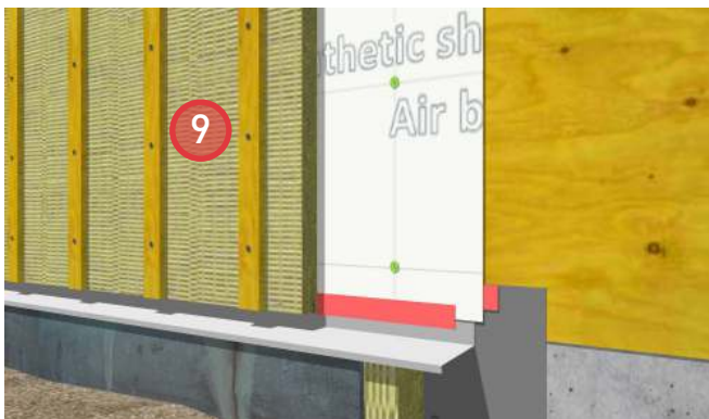
9. Install ROXUL® COMFORTBOARD™ IS. Use strapping to hold the insulation in place. Fasten the strapping to the wall. Provide bugscreens at the top and bottom of the strapping.
