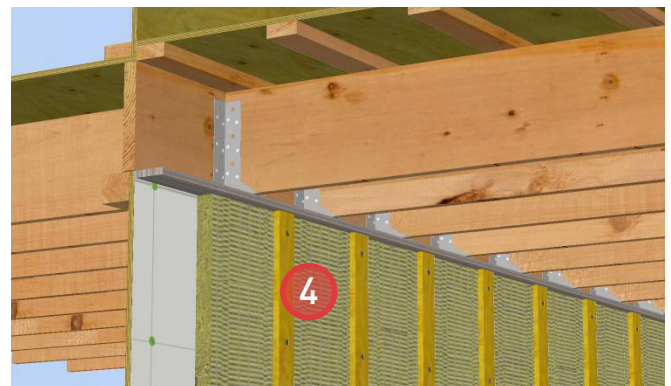
4. Install ROXUL® COMFORTBOARD™ IS and strapping with bugscreens, leaving a \frac{3}{4} " gap to ensure air barrier continuity through sheathing to rim joist interface. Suggest using a 1x4 temporary spacer board to space the insulation.
