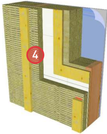
4. Install ROXUL® COMFORTBOARD™ IS and secure with strapping.
