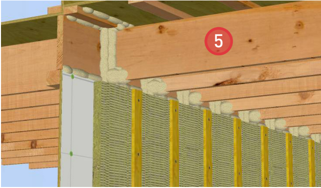
5. Remove the spacer board and install 2 lb. closed-cell spray foam or sealant at all joints in the joist cavity to maintain air barrier continuity.
