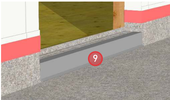
9. Install sub-sill prefinished metal flashing. Adhere to the PVC deck membrane to avoid puncture of the membrane.
