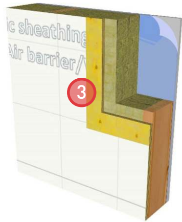
3. Install sheathing membrane.
