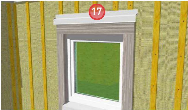
17. Install metal flashing to the strapping at the top window trim board to aid in water diversion.
