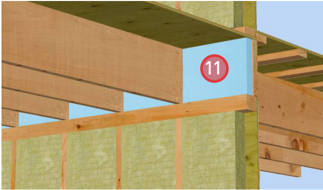
11. Install 3" rigid insulation in joist cavities. ROXUL® COMFORTBOARD™ IS and ROXUL® COMFORTBATT® can be used to meet thermal barrier protection requirements for foamed plastics.
