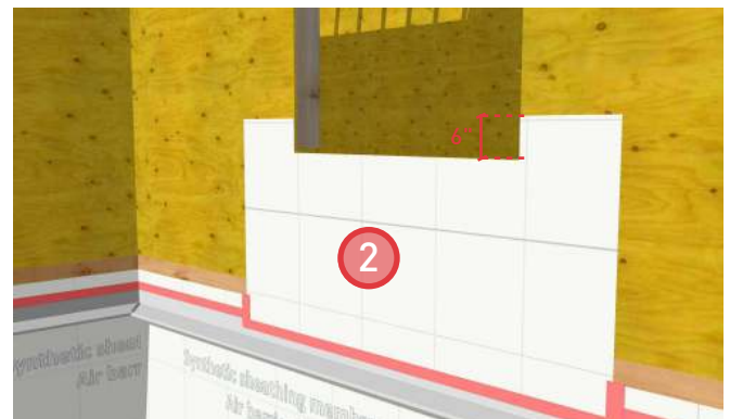
2. Install starter strip of sheathing membrane below the window rough opening. Seal the leading edge with sheathing tape.
