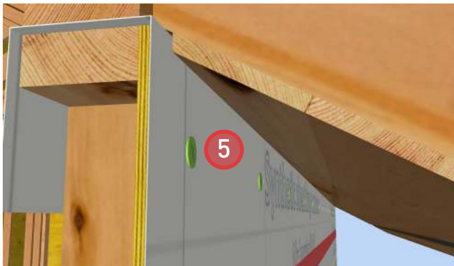
5. Install soffit material and vents.
