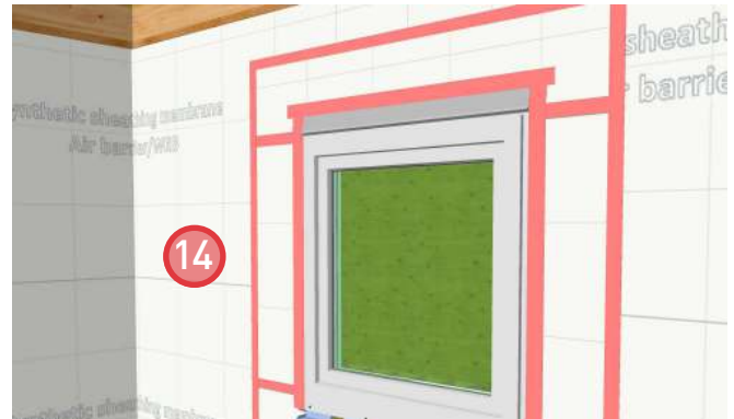
14. Install sheathing membrane. Ensure positive laps over all other layers. Seal the leading edge with sheathing tape.
