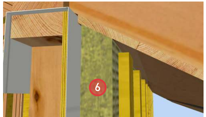
6. Install ROXUL® COMFORTBOARD™ IS and strapping to the exterior of the wall. Provide bugscreens at the top and bottom of the strapping.
