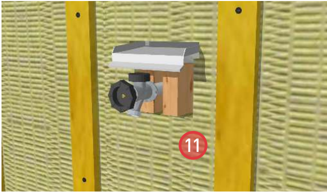
11. Install ROXUL® COMFORTBOARD™ IS and strapping. Provide bugscreens at the top and bottom of the strapping.
