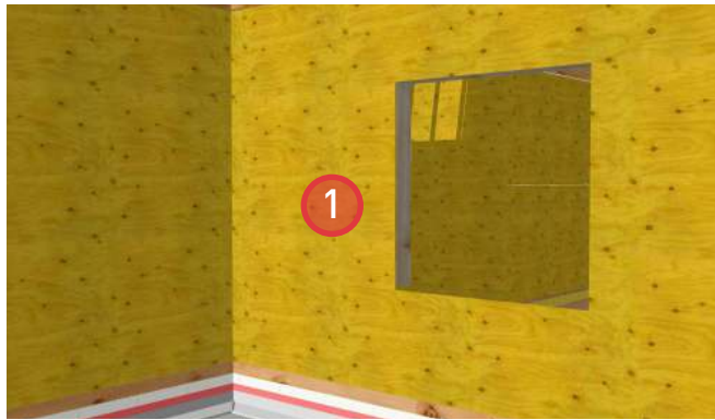
1. Typical wood frame construction at sheathing stage.
