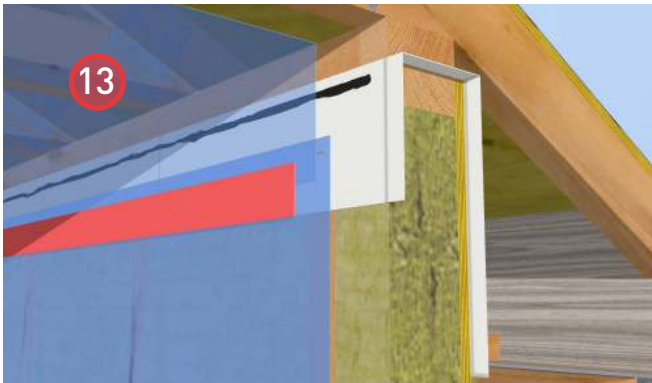
13. Install poly to the underside of the roof rafters and fasten with staples at the sealant bead to complete the air seal. Seal the leading edge of the poly with sheathing tape to maintain vapour barrier continuity.
