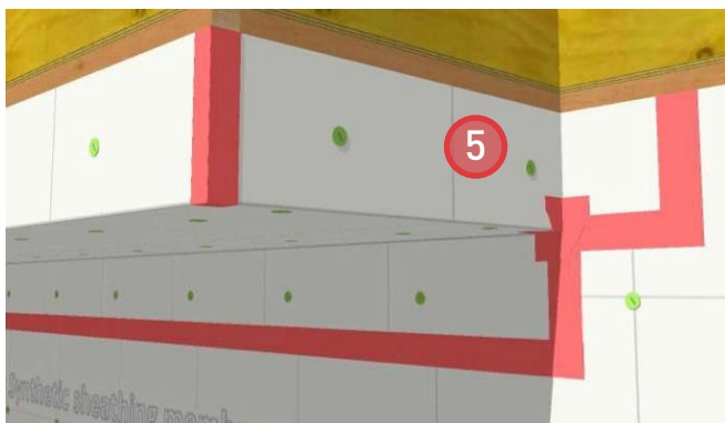
5. Install gussets constructed of sheathing tape to cover the pinholes at the inside corners.
