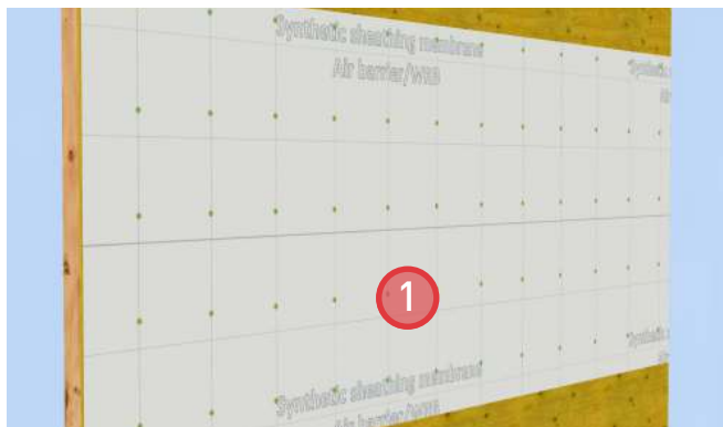
1. Install starter sheathing membrane under area where canopy will meet the wall.
