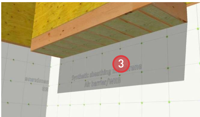
3. Install sheathing membrane. Cut to allow the membrane beside the cantilevered floor to extend up the wall 8".
