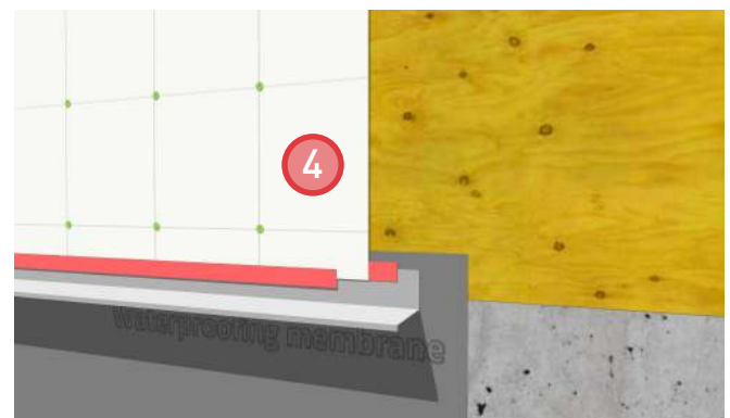
4. Install sheathing membrane and seal leading edge to the flashing with sheathing tape to complete air barrier continuity. Provide a 3/4" vision line on the flashing backleg.
