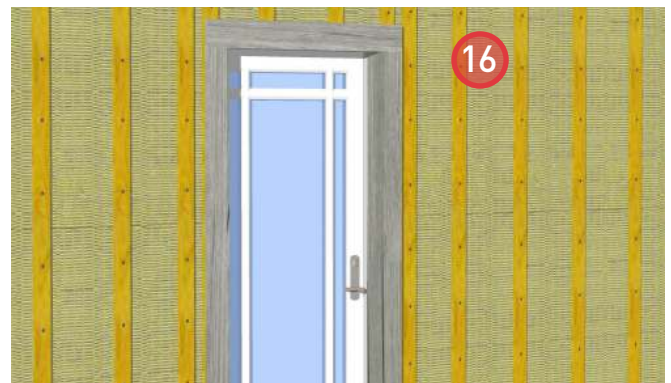
16. Install swing door trim boards.
