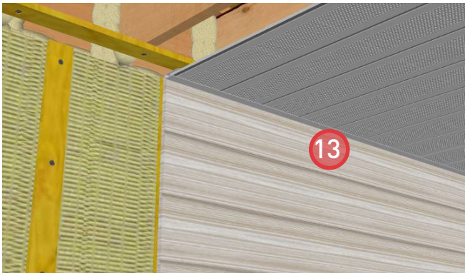
13. Install cladding and vented soffit panels below balcony.
