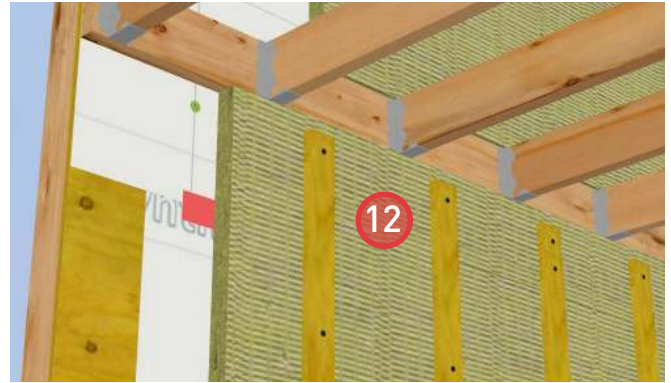
12. Install ROXUL® COMFORTBOARD™ IS and secure in place with strapping. Provide bugscreens at the top and bottom of the strapping.
