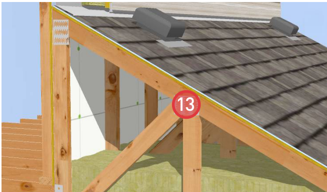
13. Install ROXUL® COMFORTBATT® in the attic space. Insulate wall adjoining attic space and occupied space with ROXUL® COMFORTBATT®.
