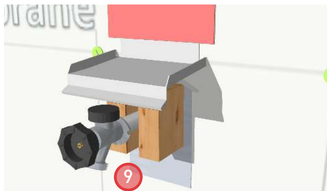
9. Install prefinished metal flashing above the hose bib and seal the leading edge with sheathing tape to provide for air barrier continuity.
