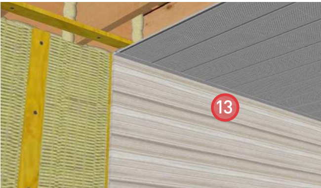
13. Install cladding and vented soffit panels to the underside of the balcony.
