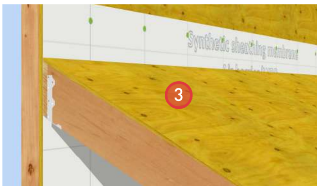
3. Install canopy roof deck material.
