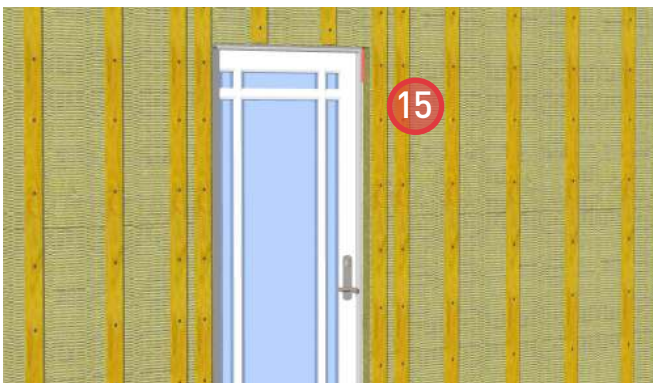
15. Install ROXUL® COMFORTBOARD™ IS and secure in place with strapping. Provide bugscreens at the bottom and top of the strapping.
