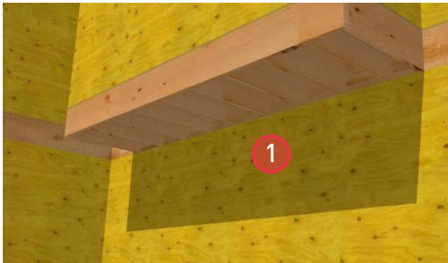
1. Typical wood frame construction at sheathing stage.
