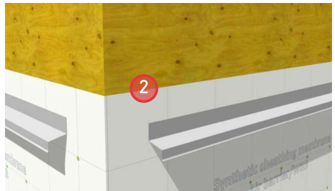
2. Install sheathing membrane and flashing.
