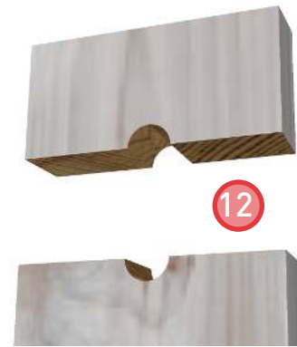
12. Create the wood face plate from dimensional lumber. The diameter of the hole in the center is equal to the diameter of pipe on the hose bib.
