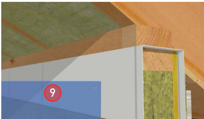
9. Install the poly sheet on the interior face of the wall. Fasten the poly to the sheathing membrane with staples at each stud.
