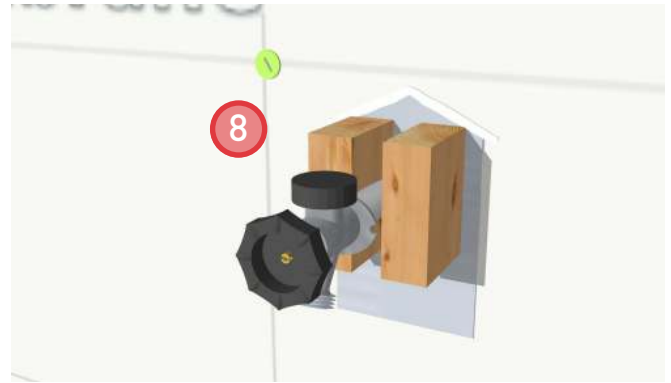
8. Install blocking to support the hose bib and onto which the face plate will be attached.
