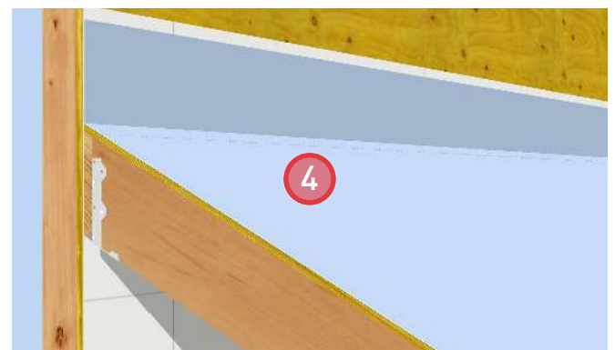
4. Install waterproof canopy deck membrane. Return the membrane 8" up the adjacent wall.
