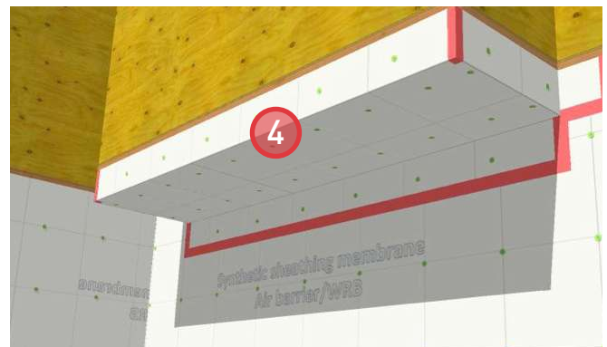
4. Install sheathing membrane along the cantilevered floor joists. Seal all leading edges with sheathing tape to maintain air barrier continuity. Fold corners on the upturn and seal the fold with sheathing tape.
