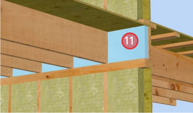
11. Install rigid insulation in joist cavities. ROXUL® COMFORTBOARD™ IS and ROXUL® COMFORTBATT® can be used to meet thermal barrier protection requirements for foamed plastics.
