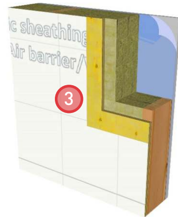
3. Install sheathing membrane.
