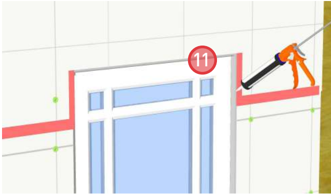
11. Install backer rod and sealant around the exterior perimeter of the door frame.
