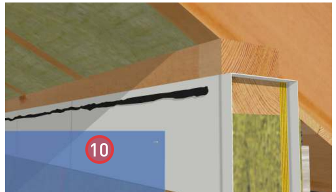
10. Install a bead of acoustical sealant on the sheathing membrane at the lower top plate to transition the air barrier from the wall to the ceiling.
