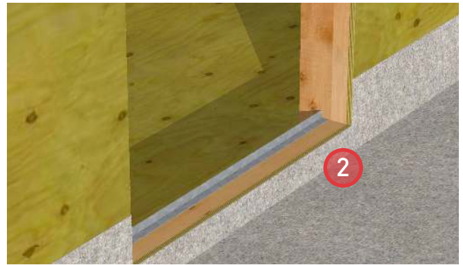
2. Install PVC balcony membrane. Extend the membrane to the height of the rough opening and elsewhere to a minimum height of 8" above the finished deck grade.
