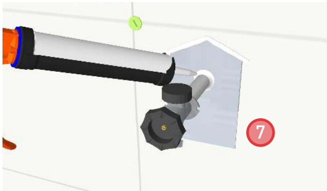
7. Apply a bead of sealant around the perimeter of the hose bib, ensuring good adhesion to the foil-faced membrane to maintain air barrier continuity.
