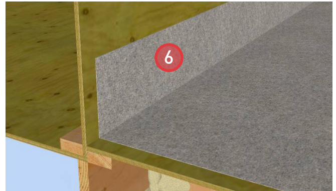
6. Install waterproof PVC balcony membrane and extend 8" up adjacent wall.
