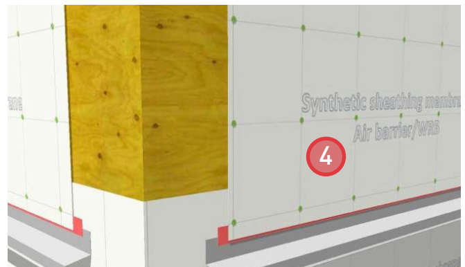
4. Install upper layer of sheathing membrane. Lap the membrane over the flashing.
