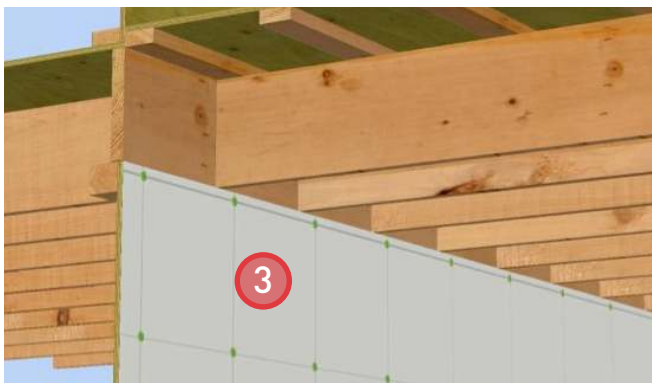
3. Install sheathing membrane and apply pressure to ensure adhesion to the sealant bead.
