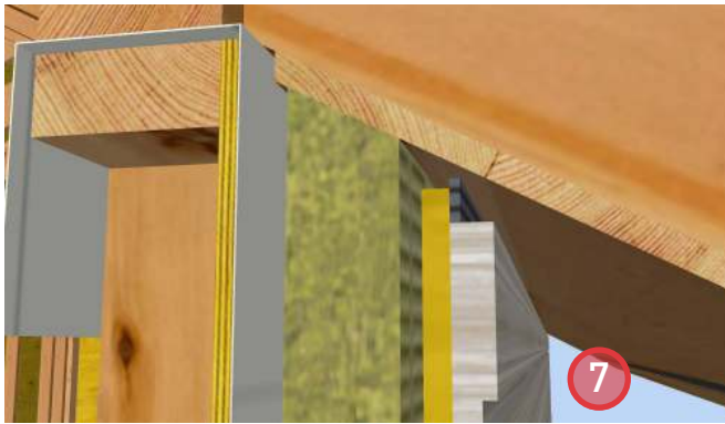
7. Install cladding. Allow for venting of the wall cavity at the top of the cladding underside of the soffit.
