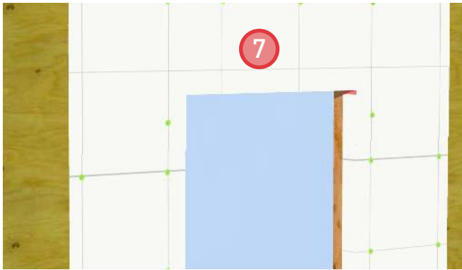
7. Install sheathing membrane at the head. Return the sheathing membrane into the rough opening.
