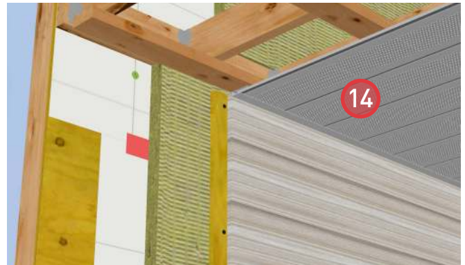
14. Install vented soffit material.
