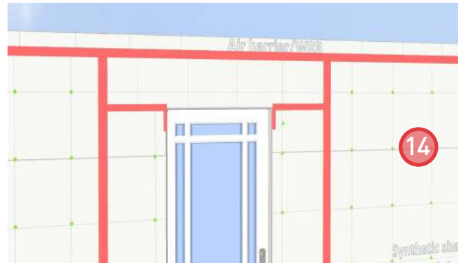
14. Install sheathing membrane from above and seal the leading edge with sheathing tape to maintain air barrier continuity. Ensure the sheathing membrane laps over membrane layers below.
