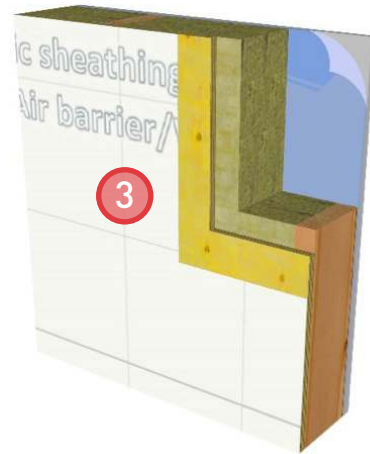
3. Install sheathing membrane.
