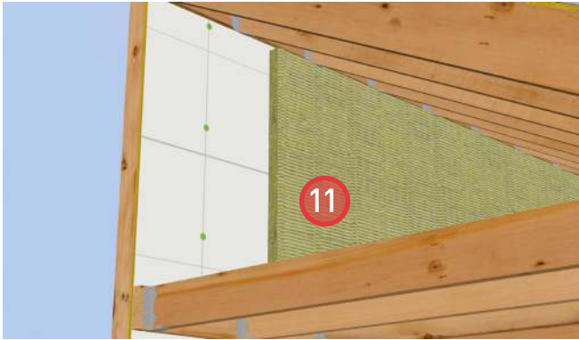
11. Install sheathing membrane below the canopy. Ensure the membrane laps under the starter strip. Seal the leading edge of the starter strip membrane with sheathing tape to maintain air barrier continuity.
