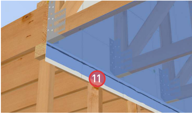
11. Install poly and seal the leading edge to the sheathing membrane with staples through the poly at the sealant bead to complete the air barrier continuity.
