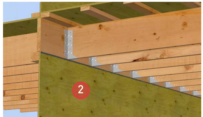
2. Install a bead of sealant along the sheathing directly below the balcony joists to provide for air barrier continuity.
