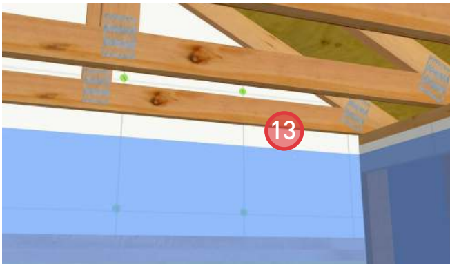
13. Install poly on the walls and fasten to the sheathing membrane with staples.
