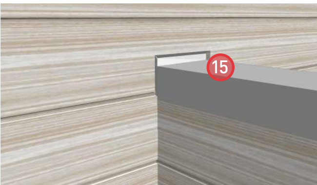
15. Install cladding. Leave a gap around the flashing to allow for sealant.
