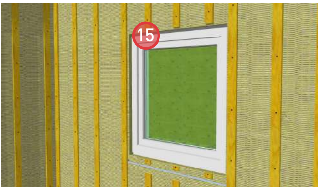
15. Install ROXUL® COMFORTBOARD™ IS and secure with strapping. Provide bugscreens at the top and bottom of the strapping.
