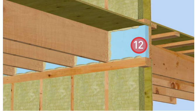
12. Install 2 lb. closed-cell spray or sealant around the perimeter of the rigid insulation to ensure air tightness and thermal barrier continuity.
