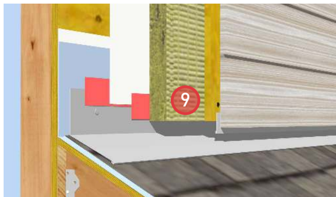
9. Install cladding and closure flashing.
