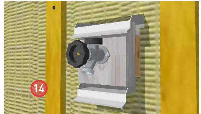
14. Install the bottom block and sill flashing. The sill flashing is fastened to the back of the bottom block.
