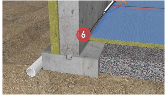
6. Install poly over the insulation and seal the leading edge to the foundation wall with acoustical sealant to maintain air barrier continuity. Seal laps in the poly with acoustical sealant and sheathing tape on the leading edge.
