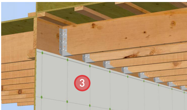
3. Install sheathing membrane and apply pressure to ensure adhesion to the acoustical sealant bead.
