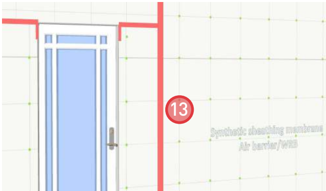
13. Install sheathing membrane to the rest of the wall. Seal the vertical leading edge with sheathing tape to maintain air barrier continuity.
