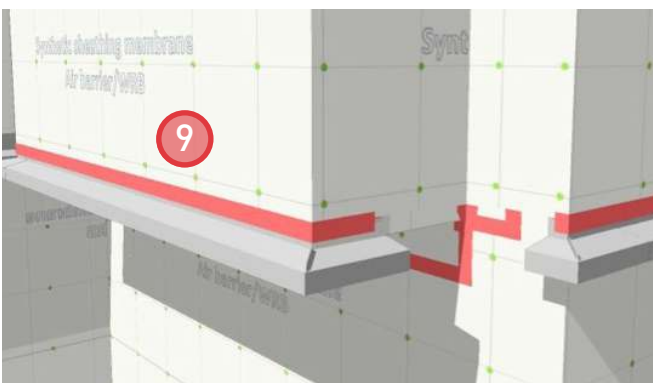
9. Seal the leading edge of the sheathing membrane with sheathing tape to maintain air barrier continuity.
