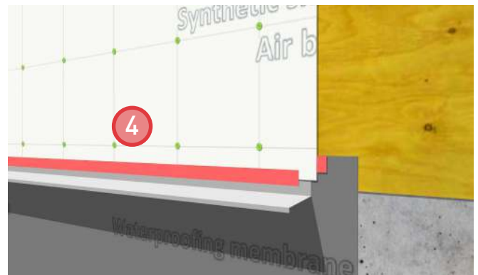
4. Install sheathing membrane and seal leading edge with sheathing tape to complete air barrier continuity. Provide a 3/4" vision line on the flashing backleg.
