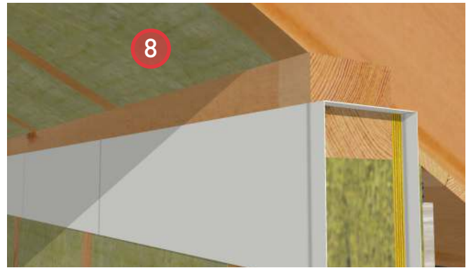
8. Install ROXUL® COMFORTBATT® in the stud cavities and roof cavity. Provide venting per building code requirements.
