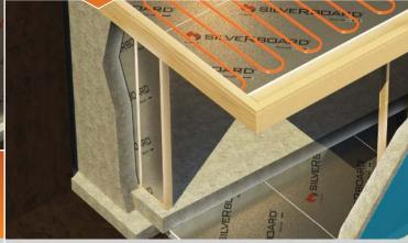
SilveRboard Acoustic is a rigid flat-sheet insulation board that offers dramatic sound control properties up to IIC 70 coupled with radiant barrier (heat reflecting) properties and R5.6 insulation for use in residential, low rise, apartments and townhouses or high-rise residential or commercial. SilveRboard Acoustic increases jobsite efficiency and reduces labor costs.
