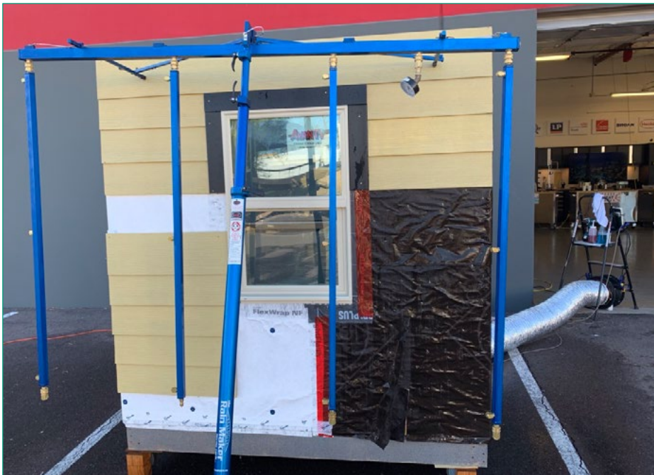
Figure 1. While adhesive flashings play a vital role in shielding seams and interfaces from water and air intrusion, their performance plays out hidden for years by exterior layers. Mock-up wall with window, ready for testing, at Construction Instruction's Phoenix, Arizona research facility. Photo courtesy Construction Instruction.
