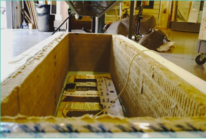
Figure 3. Heat taping testing in the oven at Construction Instruction's Phoenix, Arizona research facility. Photo courtesy Construction Instruction.
