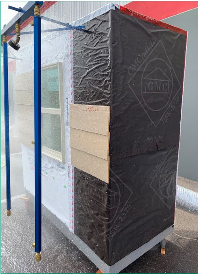
Figure 5. Testing a mock-up enclosure for performance during a rain event. Where and how water can penetrate an assembly, and how that assembly dries, are critical questions for every wall. Photo courtesy Construction Instruction.
