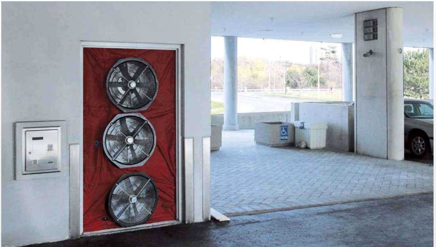
Typical blower door test at multi-story building
