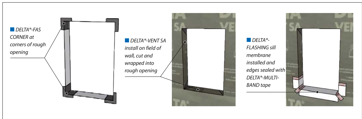
Figure 3: Sub-sill flashing below all window and door openings is a critical component to ensure resistance to rain penetration.
