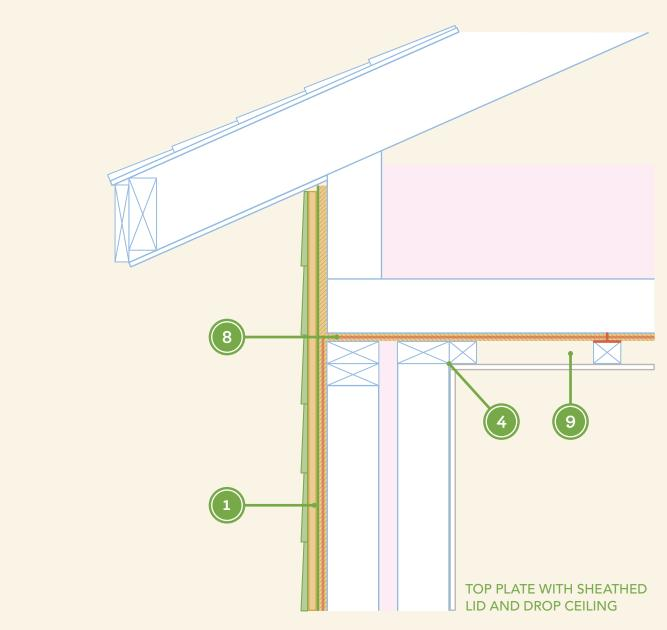
Cladding/siding = --Rain screen batten = Rigid insulation = 💳 Wall exterior sheathing with weather-resistive barrier = 📼 Interior finish/wallboard = Tape, gasket or sealant = – Insulation = High-density spray foam = Concrete =
