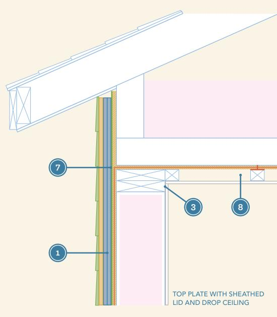
Cladding/siding = Rain screen batten = Rigid insulation = 💳 Wall exterior sheathing with weather-resistive barrier = Interior finish/wallboard = Tape, gasket or sealant = • Insulation = High-density spray foam = Concrete =
