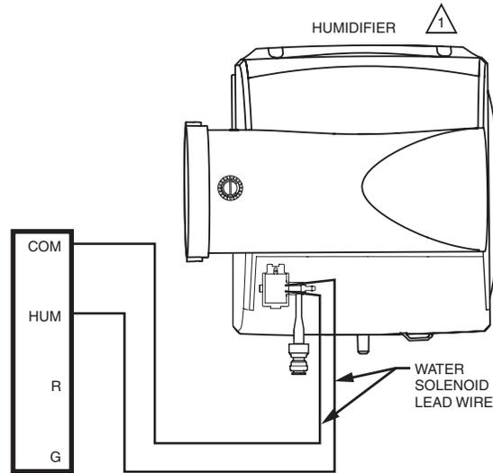
1 WIRING DIAGRAM ASSUMES THE USE OF EQUIPMENT-SPECIFIC COMMUNICATING THERMOSTAT CONTROLLING THE HUMIDIFIER.
