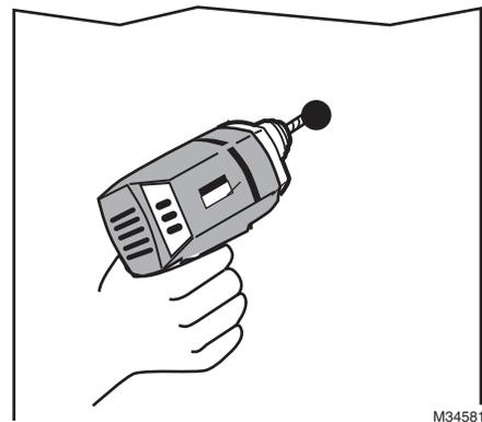
Find your mark and drill a 1/2 in. hole in the duct. This is where the duct tube will be inserted to capture air.
