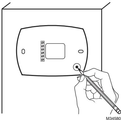
Hold the wallplate up to the desired location on the duct and make a mark inside the duct tube hole.
