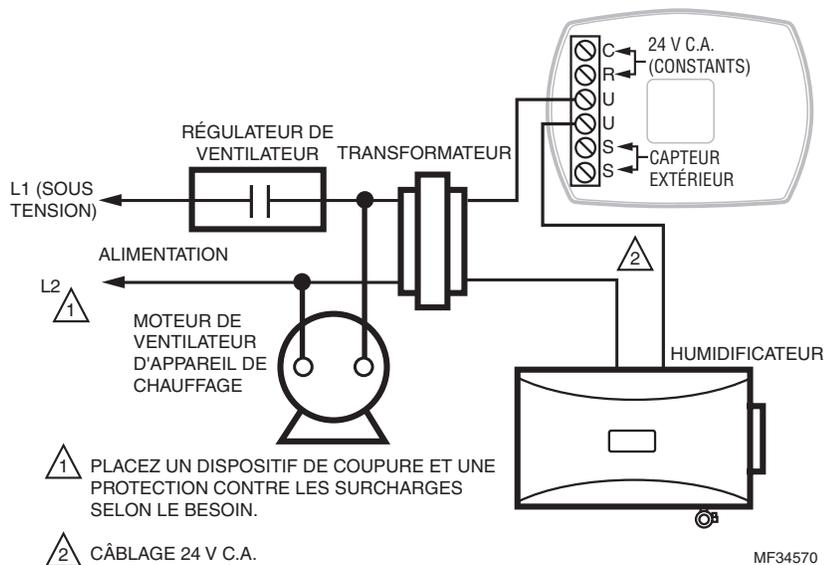
1 PLACEZ UN DISPOSITIF DE COUPURE ET UNE PROTECTION CONTRE LES SURCHARGES SELON LE BESOIN.
