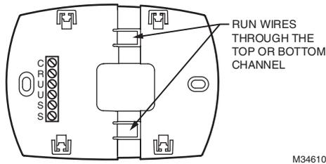
Run wires through the top or bottom channel on the back plate when duct-mounted. If installing like a thermostat on a wall, run the wires through the back.
