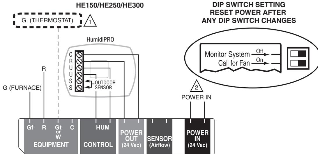
1 ONLY NEEDED IF SYSTEM'S THERMOSTAT DOES NOT ISOLATE Y FROM G. IF NEEDED, BREAK THE THERMOSTAT G TO SYSTEM G CONNECTION AND ROUTE THROUGH HUMIDIFIER AS SHOWN.
