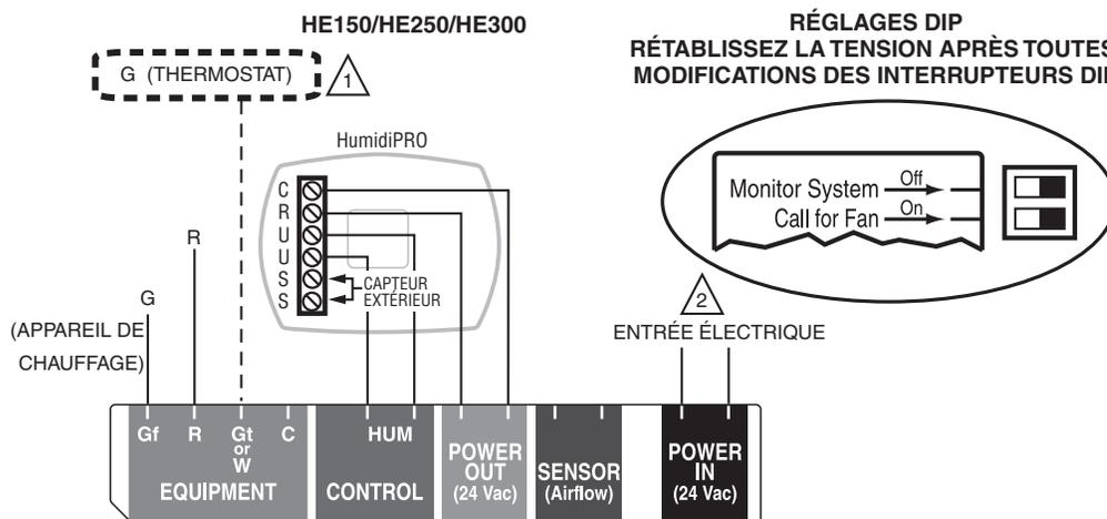
1 UNIQUEMENT REQUIS SUR LE THERMOSTAT DU SYSTÈME N'ISOLE PAS Y DE G. SI NÉCESSAIRE, COUPEZ LA CONNEXION DU G DU THERMOSTAT AU G DU SYSTÈME ET ACHÉMINÉZ PAR L'HUMIDIFICATEUR COMME ILLUSTRÉ.
