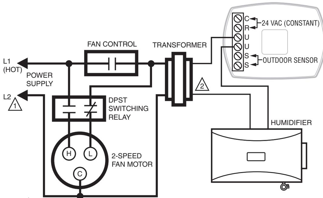
1 PROVIDE DISCONNECT MEANS AND OVERLOAD PROTECTION AS REQUIRED.
