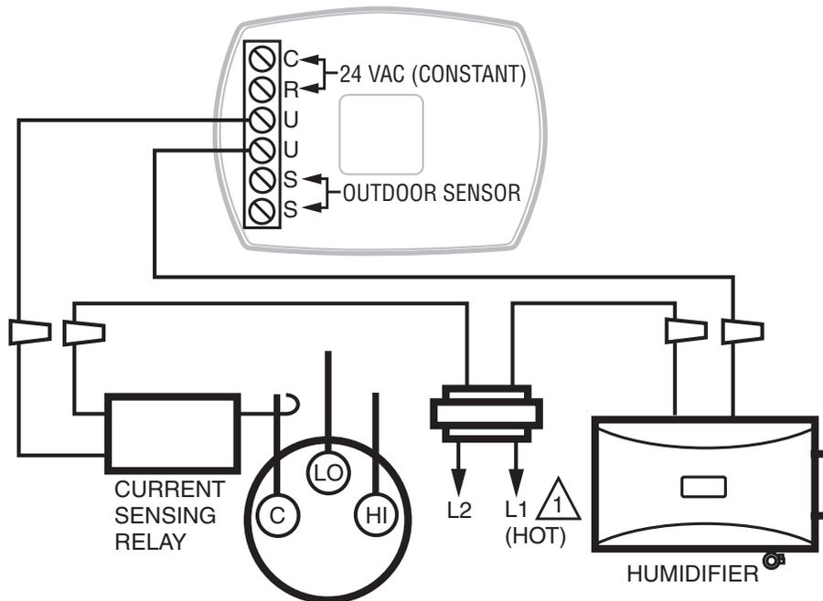
1 PROVIDE DISCONNECT MEANS AND OVERLOAD PROTECTION AS REQUIRED.
