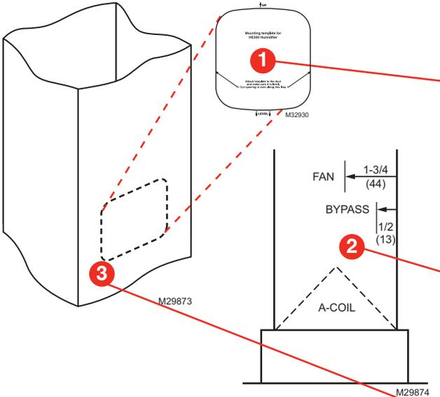
Position the template on the duct.
