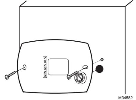
Secure the wallplate to the duct with sheet metal screws (provided).
