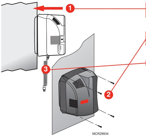
Slide the Fan model evenly into the duct hole. Verify the humidifier is level.
