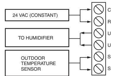
NOTES: C AND R MUST BE CONSTANT 24VAC! RECOMMENDED TO WIRE TO FURNACE/AIR HANDLER CONTROL BOARD.
