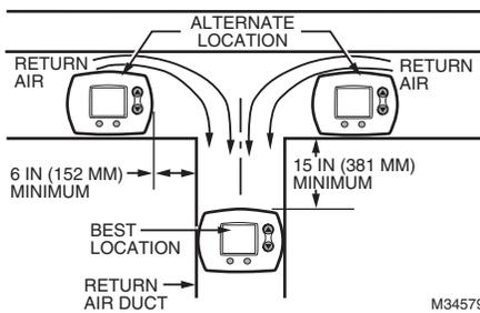
**Warning: Product must be mounted on the RETURN side of the duct for proper RH% sensing.**
