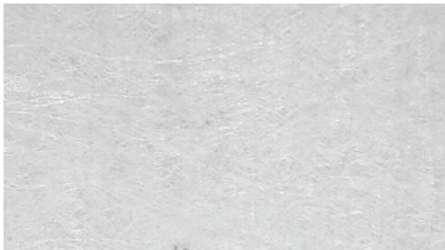
Tyvek® HomeWrap®: no mold growth after 75 days.
