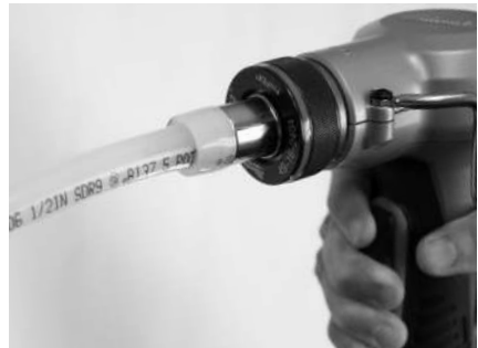
Figure 6-4: Expand until ring is snug against expander head
