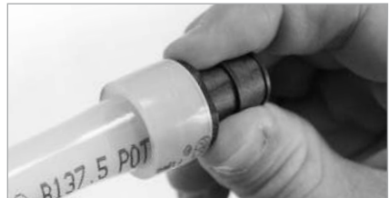
Figure 6-8: Ensure tubing and ring seat against shoulder of fitting
