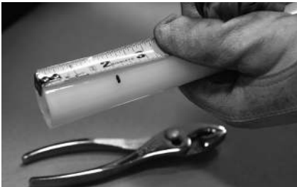
Figure 6-16: Measure 2" of tubing
