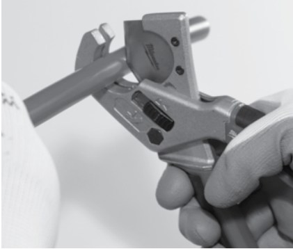
Figure 3-6: Square cut the pipe
