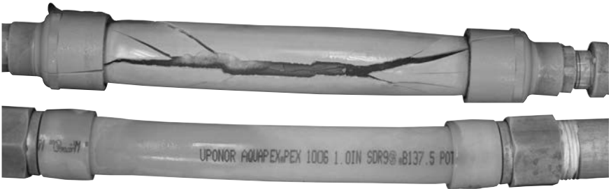
Figure C-2: CPVC vs. PEX freeze test
