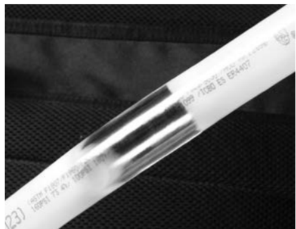
Figure C-1: Reforming kinked piping
