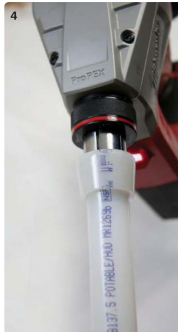
Expansion with Milwaukee M18 ProPEX Expansion Tool
