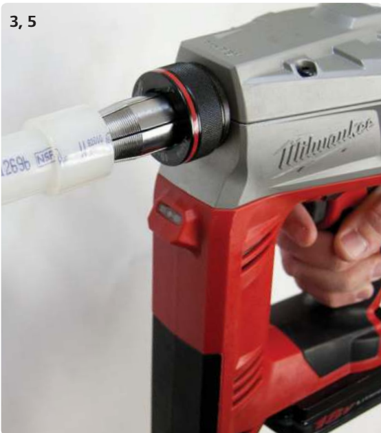
Expansion with Milwaukee M18 ProPEX Expansion Tool
