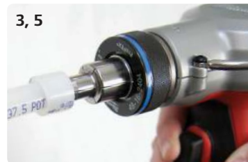
Expansion with Milwaukee M12 ProPEX Expansion Tool
