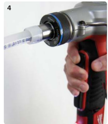
Expansion with Milwaukee M12 ProPEX Expansion Tool
