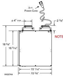
NOTE: ALL UNITS PORTS WERE CREATED TO BE CONNECTED TO DUCTS HAVING A MINIMUM OF 4" DIAMETER, BUT IF NEED BE, THEY CAN BE CONNECTED TO BIGGER SIZED DUCTS BY USING AN APPROPRIATE TRANSITION (E.G.: 4" DIAMETER TO 5" DIAMETER TRANSITION).
