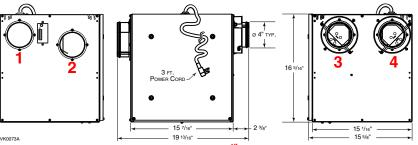
NOTE: ALL UNITS PORTS WERE CREATED TO BE CONNECTED TO DUCTS HAVING A MINIMUM OF 4" DIAMETER, BUT IF NEED BE, THEY CAN BE CONNECTED TO BIGGER SIZED DUCTS BY USING AN APPROPRIATE TRANSITION (E.G.: 4" DIAMETER TO 5" DIAMETER TRANSITION).
