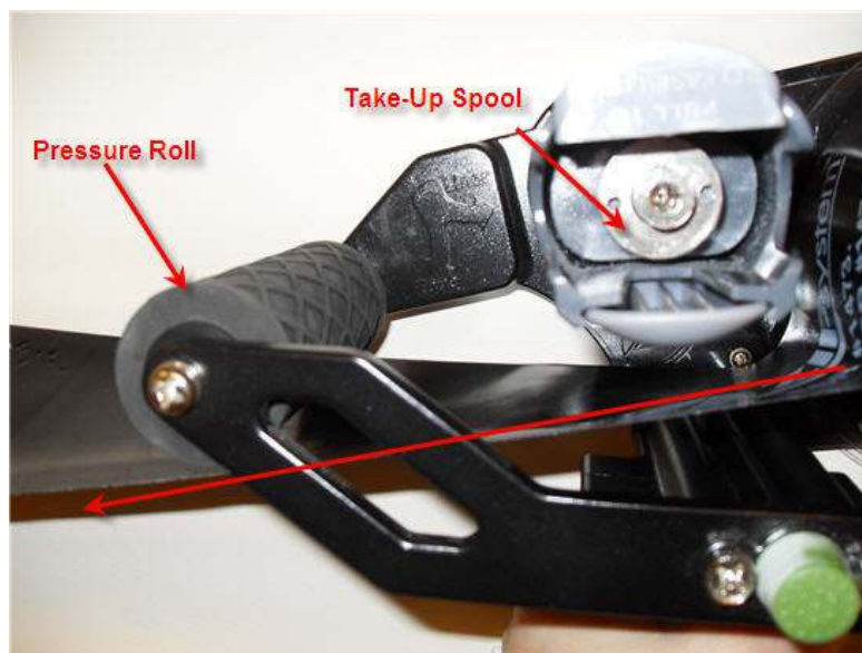
Picture 2. Feed the tape under the take-up spool and pressure roller
