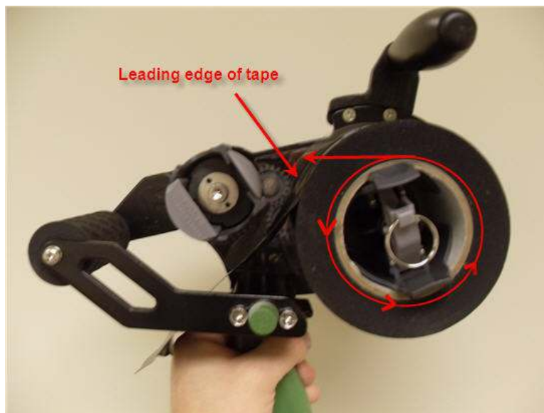
Picture 1. Loading tape roll on unwind spool
