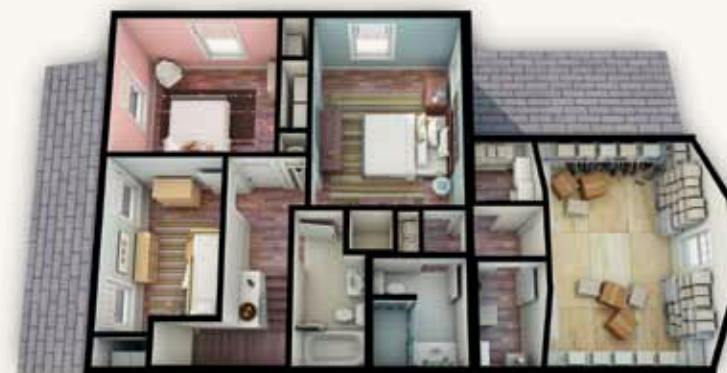
SECOND FLOOR In this example, the second floor is packed with three bedrooms, two baths, and an unfinished storage area, but the plan is flexible. If the first-floor suite is used as a master suite, the second floor could have larger bedrooms and a single shared bath. For more living space, the attic is just waiting to be colonized.
