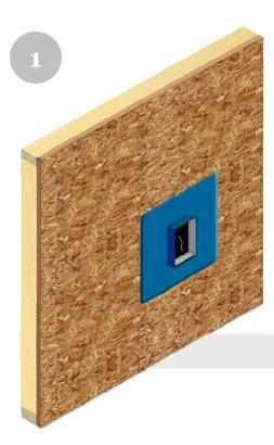
Slide Quickflash® panel onto electrical box firmly pressing panel against the wall or studs.
