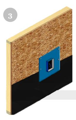
Slide the weather resistant barrier underneath the Quickflash® panel to the bottom of the electrical box.
