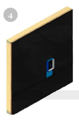
Install the weather resistant barrier carefully cutting an opening around the protruding electrical box, over the top of Quickflash® panel using shingle style method extending to the bottom of flashing panel or further.
