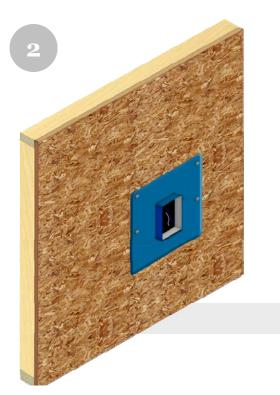
Using non-corrosive fasteners, secure the Quickflash® panel to the structure from the midpoint of the panel to the top.
