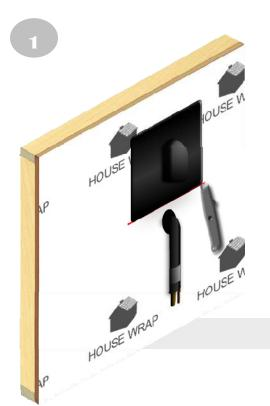
Using the Quickflash® panel as a guide, mark the length of the panel plus 1/4" on each side 2" above penetration onto the WRB and using a utility knife, cut a slit along the mark.
