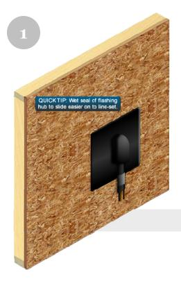
Slide Quickflash® panel onto line-set firmly pressing panel against the wall or studs.
