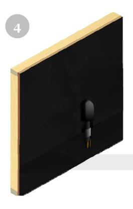
Install the weather resistant barrier carefully cutting an opening around the protruding line-set, over the top of Quickflash® panel using shingle style method extending to the bottom of the panel or further down.
